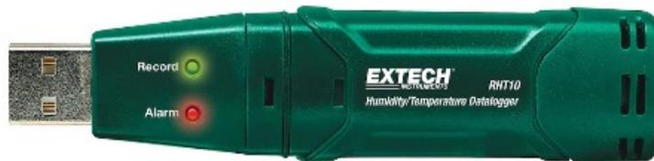
**Extech**, a maker of electronic test instruments, will soon deliver this RHT10 model to Canada. Mount it in any location where moisture and heat are of concern. Values for both will be recorded in memory, transferable when plugged into a Windows computer. Should moisture or heat reach a threshold, this device will sound and alarm.
